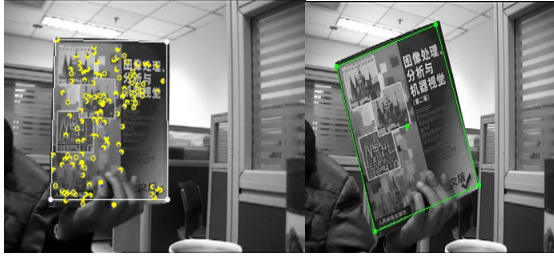
Fig. 1. The correspondence between the vertices according to the homography matrix
