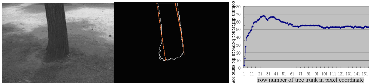
Fig. 3. A frame showing some tall vertical structure(left), a edge extraction image by using LOG operator and thinning algorithm, brown indicates the least squares line fit of edge points (middle), and tree trunk column difference between the same raw, which shows the slope of Least squares line fit (in brown) is almost equal (right)
